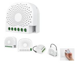
It activates and deactivates the users to which it is connected and measures consumption
