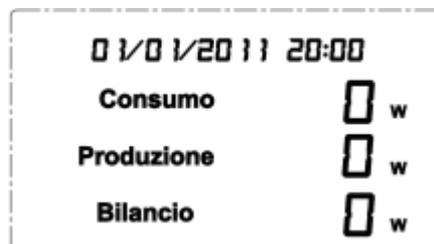
In case the controller is powered off due to power cut or battery has been used up, the data will not be lost.
