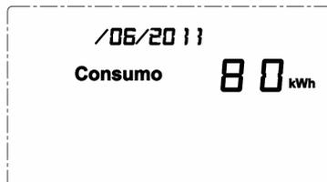
To view the history data of home electricity consumption for the last 30 days, please press the UP button on the controller and hold it for about 3 seconds under normal working conditions. When below display (assuming current month is June of 2011), release the UP button and use the UP button or DOWN button to adjust to the past other days.
