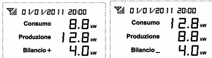
The other display is as photo below (can also be + or -, only one photo for reference). The first line is the forecast cost of next hour of home electricity consumption based on current power. The second line is the forecast yield of next hour of solar output based on current power. The last line is the balance = Solar output yield - Home consumption cost.
