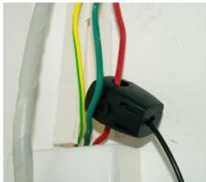
The Sensor Clamp immediately starts to detect the current and the monitoring system starts to monitor the electricity output of the home solar plant.
