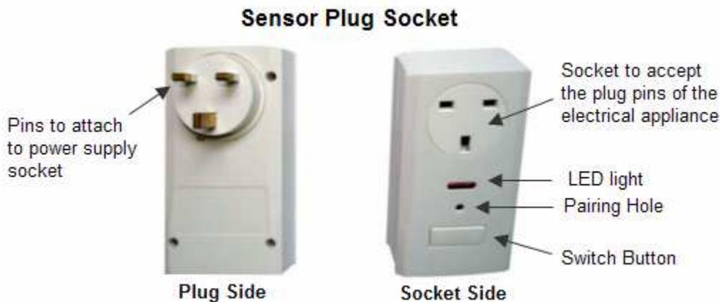
Locate an electrical appliance that is to be monitored and controlled. Attach the plug of the appliance to one Sensor Plug Socket. Then attach the Sensor Plug Socket into the power supply socket nearby.
