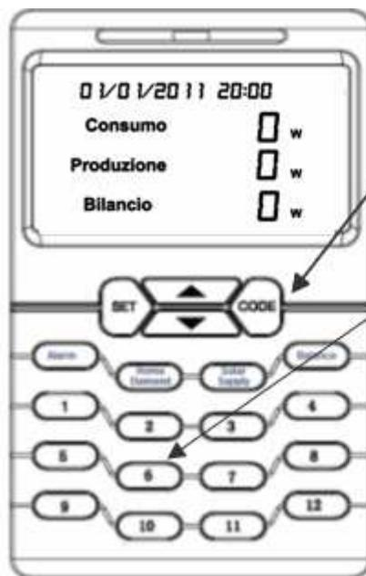
Press the "CODE" key and hold it for 3 seconds until all numbered buttons flash, then select one numbered button, for example button 6, and press it shortly. This numbered button will be used to monitor and control the Sensor Plug Socket to be paired.
