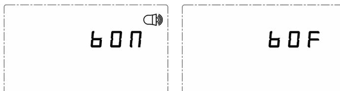
2 seconds after switching, the LCD screen will return to normal display automatically. If the buzzer is set on, the buzzer icon will always stay on the right top corner.
